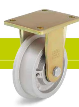
**Brackets:** BS series - Particularly rugged welded steel construction, with reinforced fork for an improved absorption of axial forces. Bolted wheel axle. Zinc-plated, yellow-passivated, Cr6-free. Bracket overview: Page 68 Top plate drawings: Page 77 and 78
