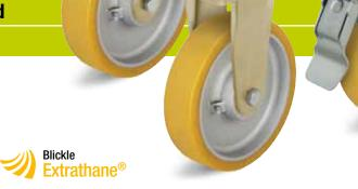
Brackets: LS/BS series - Particularly rugged welded steel construction, swivel bracket with axial grooved ball bearing DIN 711 and tapered roller bearing DIN 720 in the swivel head, dust and splash-proof, fitted grease nipple, bolted and secured with a welded very strong central kingpin. Bolted wheel axle.
