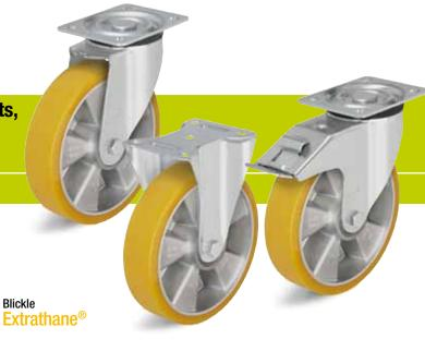
Wheels: ALTH series - Tread: Made of high-quality polyurethane-elastomer Blickle Extrathane®, 92° shore A, light brown, non-marking, non-staining. Wheel centre: Made of die-cast aluminium. Bearing type: Two pressed-in ball bearings. Detailed description: Page 246 and 48
